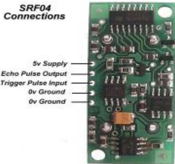
Fig 4.11 Pin configuration of ultrasonic sensor module
